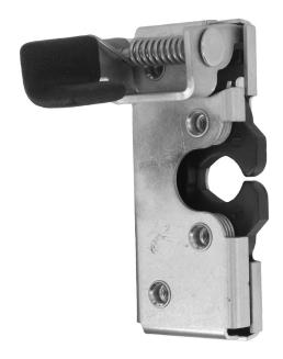
This two rotor latch is designed for medium to heavy-duty applications for on or off-highway compartments and access panels. It features a coaxial trip mechanism for applications where it is desirable to provide additional support to the trip lever with a single position latch.
